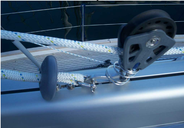
Incorrect position – will scratch the boom
